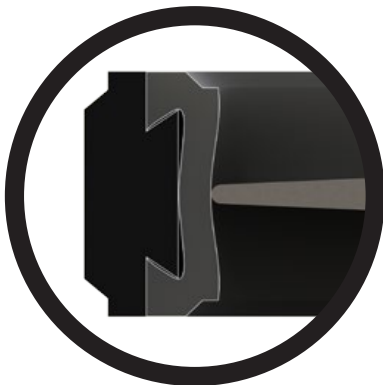
Above: Booted seat bulging around disc contact points
